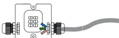
Use waterproof junction box (not less than IP65) to connect the power cord or make sure the wires with watertight treatment.
