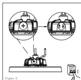
3. Open the sealing cover on top of the driver, turn off the power before adjusting the colour temperature and power, adjust the required colour temperature and power according to the prompts on the shell, in order to prevent water leakage, please tighten the sealing cover after adjustment. (see fig.3)
